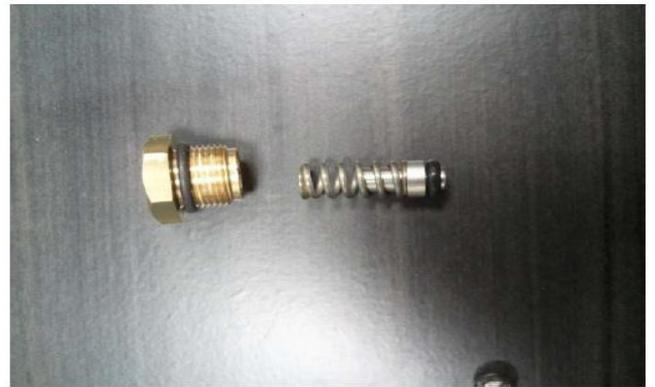
5. Re-insert spring with the shutter back to the valve housing, positioned as shown above.
