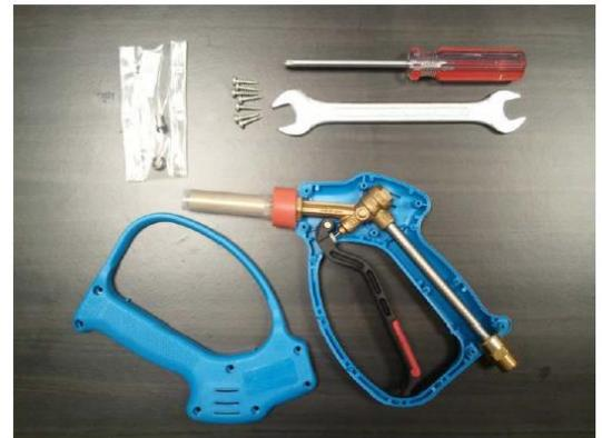
2. With a 17mm wrench, remove the brass plug on top of gun piping.
