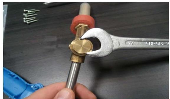
3. Pull the spring and the ball bearing. Check for wear and tear of O-rings and replace as necessary.
